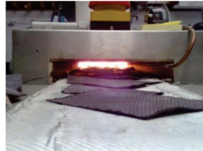
Recycling carbon fibers (left and right) and hybrid microwave conveyor ovens
